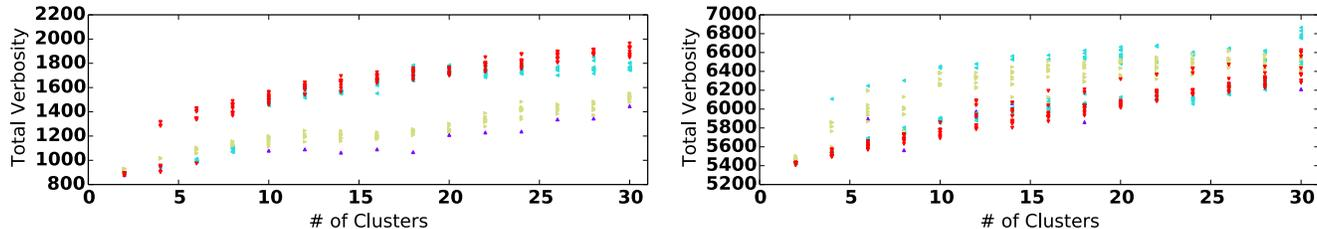
(b) Total Verbosity v. Number of Clusters (Left: PocketData, Right: US Bank); We offset Y-axis by Verbosity of the naive encoding without clustering (i.e., the total number of distinct features in the log) to show the change.
